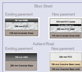
FIGURE 1 Existing and New Pavement Structures
